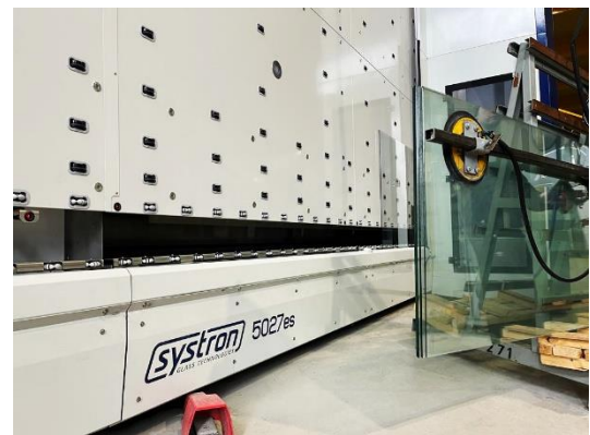
Fig. 5: Exactly the right size for Jaakko-Tuote Oy, the seaming and grinding machine systron 5027es.
