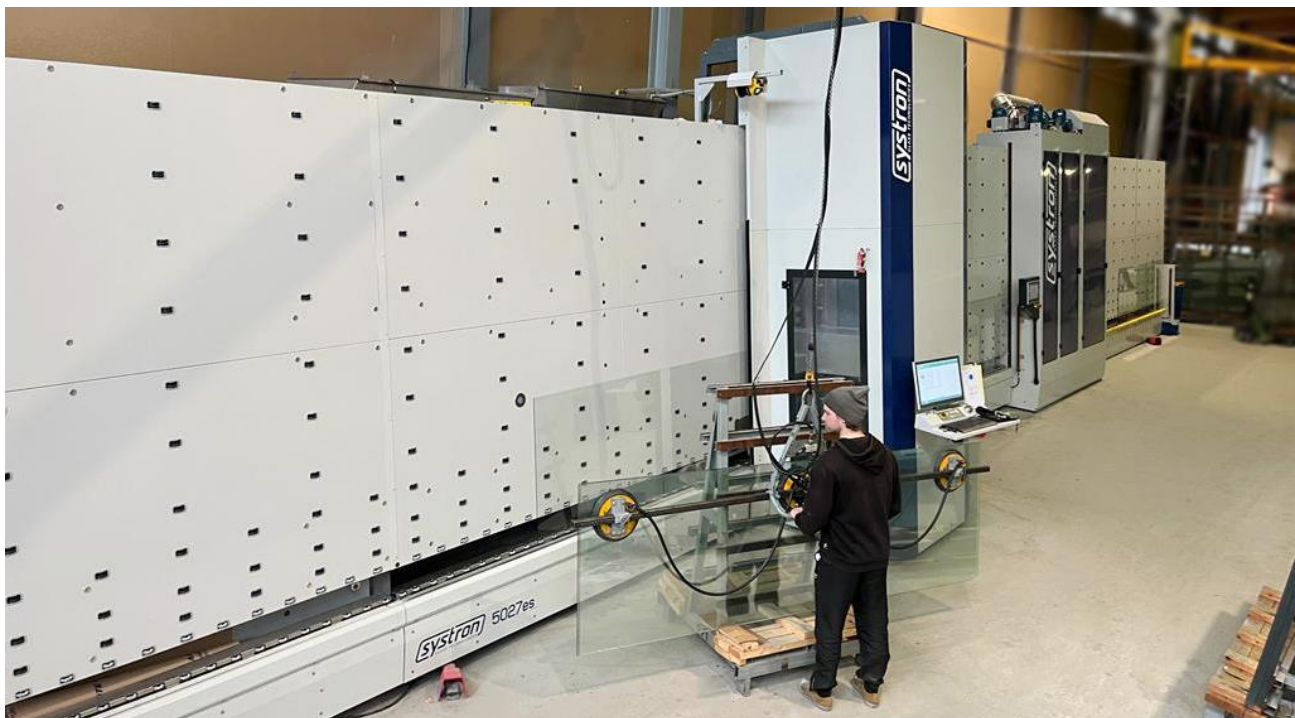
Fig. 1: The systron 5027es can seam and grind glass panes with 5m length.
