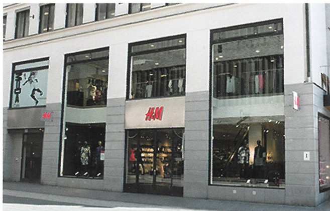
Commercial premises, Stockholm, 2007. Laminated glass 10+10 clear 1.52, ground edges, size 3125 x 5827 mm.
