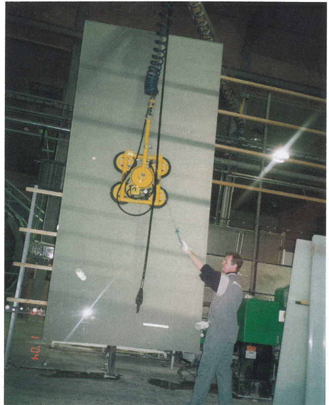
Transfer of large glass sheet to vertical polishing machine.
