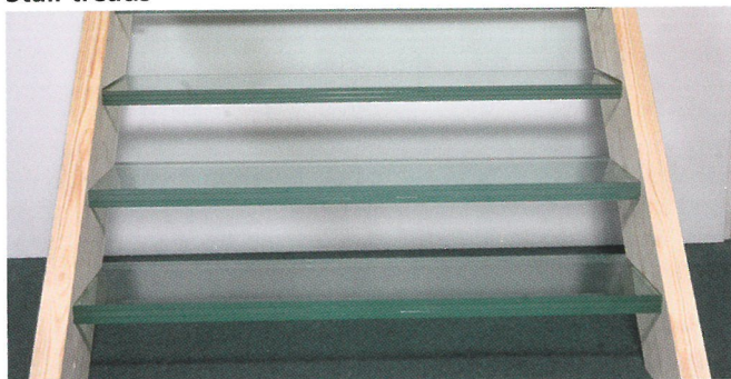
Point loading on stair treads, freely supported on two edges, width 280 mm, span 1000 mm
